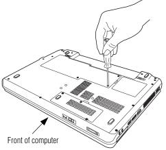
(Sample Illustration) Removing the memory module slot cover
